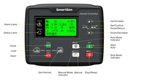
Fig.1 - HGM6110LT Front Panel Indication
